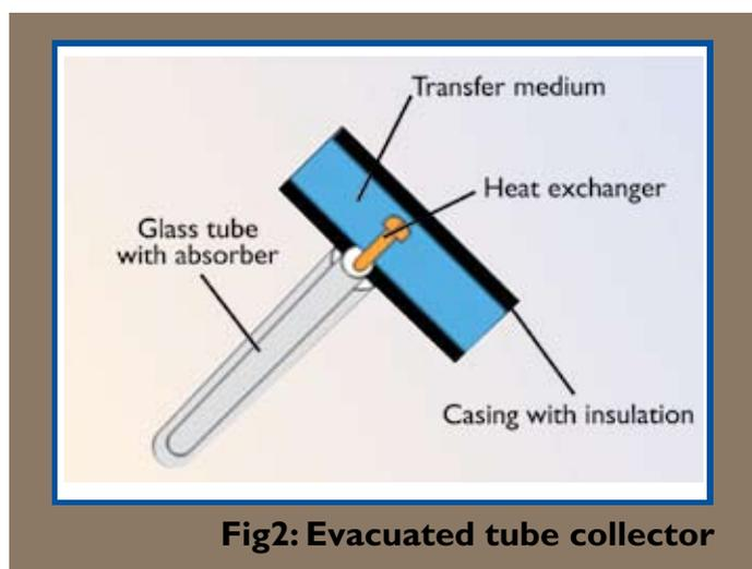
**Fig2: Evacuated tube collector**
